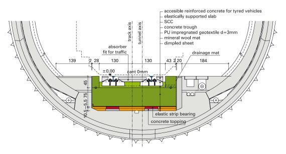
The slab provides a finishing surface with millimetre accuracy. This allows easy and accurate installation without on-site drilling of additional equipment such as noise absorbing slabs, trafficability slabs, buffer stops, track magnets and guard rails.
