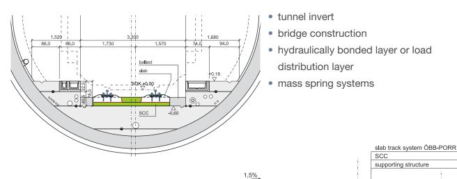
Transition areas from ballast to slab track are carried out according to the Catalogue of Specifications for Slab Track or in accordance with the ÖBB regulation RZ no.17220. The ballast area is strengthened in sections by using synthetic resin.
